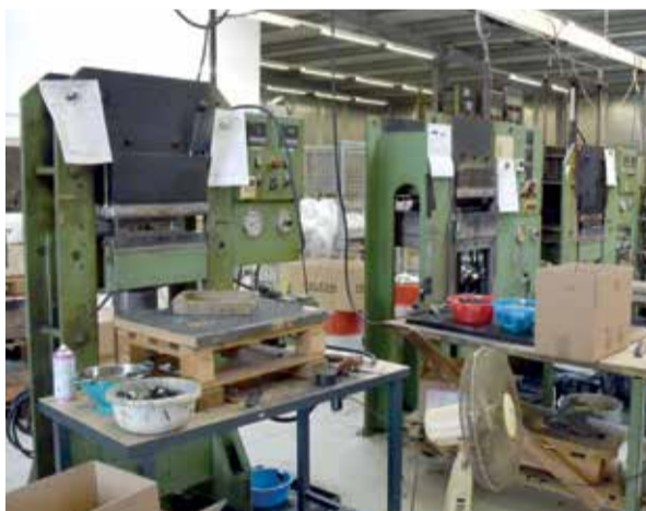
Existing compression presses
