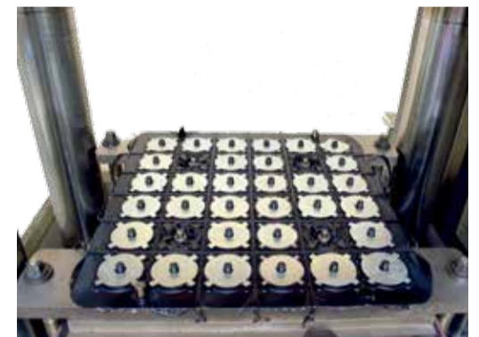
EMV rubber parts, made on a MAPLAN injection moulding machine with a pressing process
