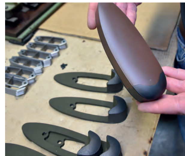
The recoil pad: A composite part made of hard rubber, stainless steel and soft rubber.
