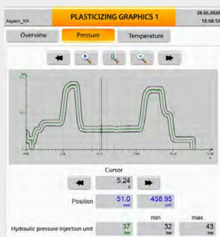
Fig 2. Pressure progression with generated envelope curve for tolerance monitoring.
