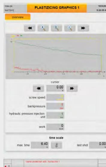
Fig 1. Overview page "Plasticizing" with graphic display of process parameters.
