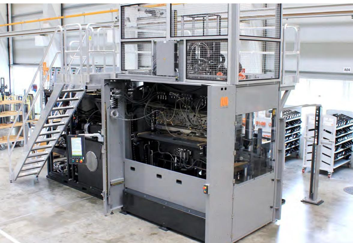
The new MAPLAN vertical machine series SPECIAL<sup>+</sup> MR is Stable, accurate and modular and suitable for many challenging applications involving Large size rubber parts with close tolerances.
