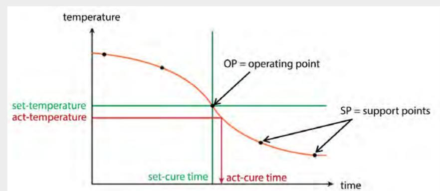
Fig.3 MAP.compensate determines a trajectory based on up to 10 mixture-specific and temperature-dependent heating times. These form the ideal basis for targeted heating corrections of environmental operating point deviations.
