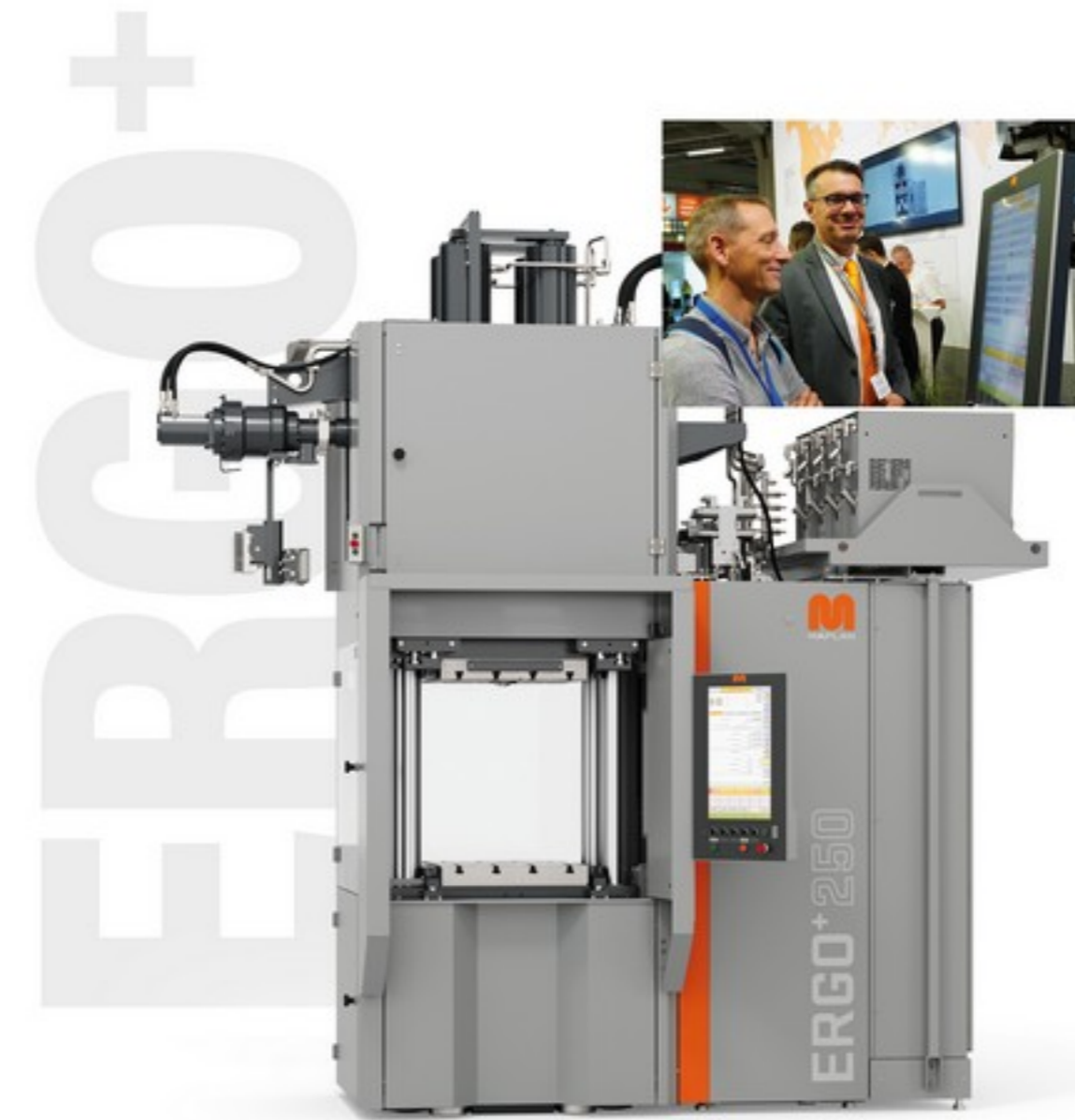
The ERGO+ 250 will be presented this year with an easily accessible MAP.fifo ergo injection unit with all FIFO advantages and ergonomic in-feed height.
