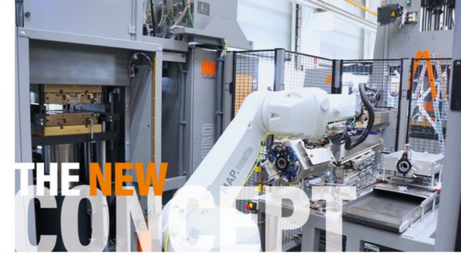
The new MAP.mate 6-axis robot in use in a fully automatic MAP.autocell
