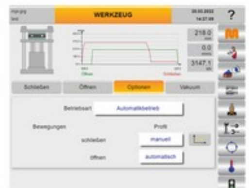
Fig 2: Tool opening and closing curves. Here: Red curve corresponds to automated closing depicted in Fig. 1.
