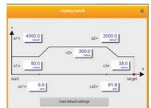
Fig 1: Closing speed settings. Here: Automatic approach of set maximum speed, automated braking until closing speed of 40.0 is reached.
